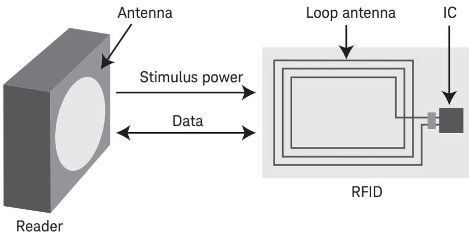
Figure 1. An overview of an RFID system
